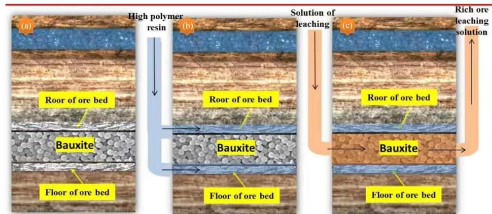
**Figure 13.** Schematic diagram of water pollution prevention with polymer resin infusion. (a) The stratigraphic procedure; (b) Schematic diagram of polymer resin filling; (c) In-Situ Leaching Mining after resin filling.
