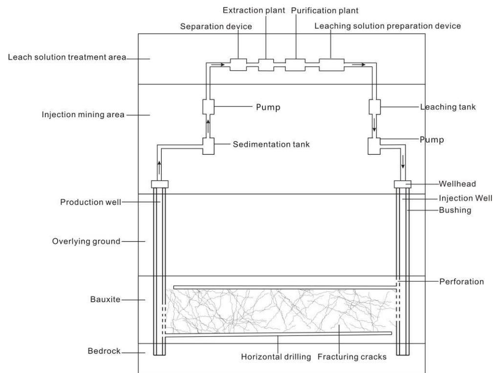
**Figure 11.** In-situ leaching of bauxite mining concept map.
