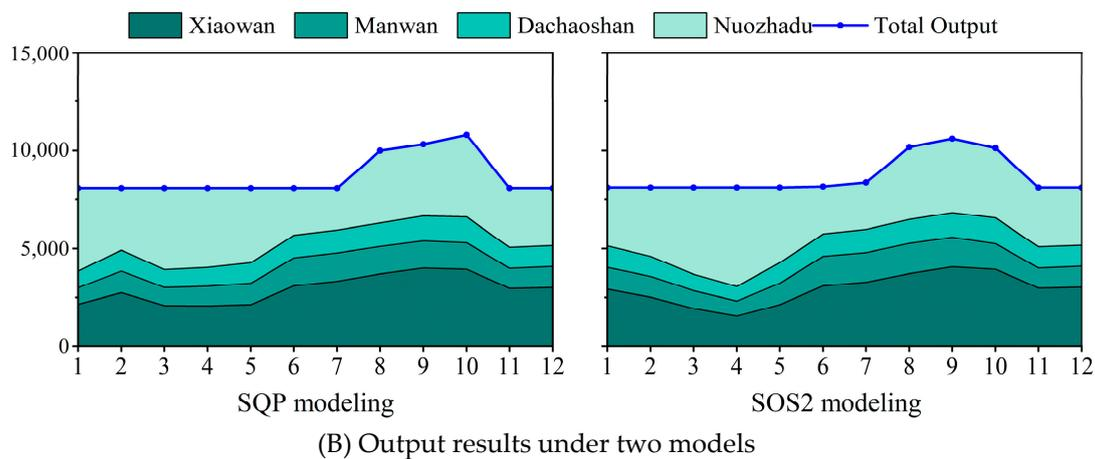
**Figure 4.** Comparison of scheduling results between two models.
