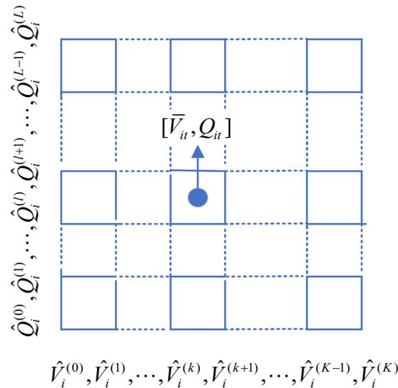
Figure 1. Gridding for piecewise linearization.
