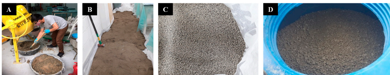
Figure 2. Preparation of mortar: (A) mixing, (B) curing, (C) crushed mortar granule, and (D) the mortar layer in the pilot plant.
