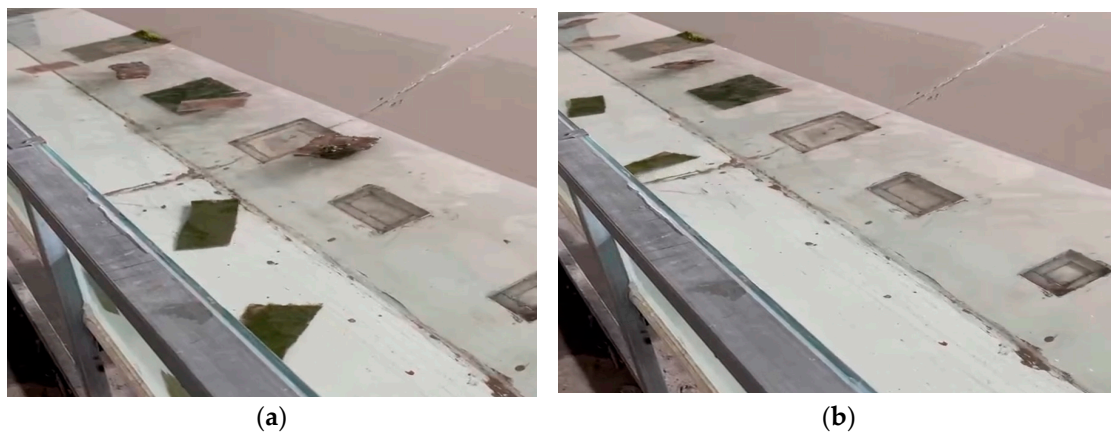
Figure 3. The transport form of epipelagic algae group at Q = 102.04 \text{ m}^3/\text{s} : (a) the state of transport in the early time; (b) the state of transport in the late time.
