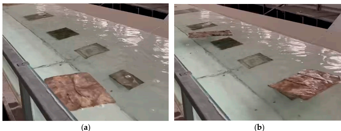
Figure 5. The transport form of epipelagic algae group at Q = 301.69 \text{ m}^3/\text{s} : (a) the state of transport in the early time; (b) the state of transport in the late time.
