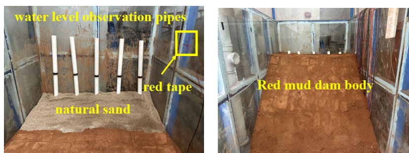
Figure 2. The water level control system.
