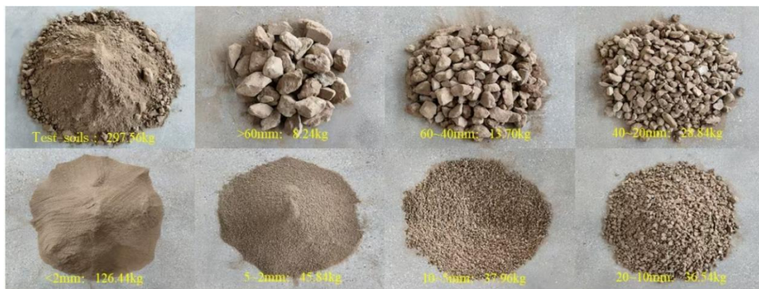
Figure 5. Characteristics of particle size distribution of bulk soil material.
