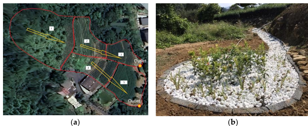
Figure 4. The studied tea farm (a) the surface flow direction and (b) the bioretention cell. Arrows indicate the direction of water flow, and numbers represent the sub-drainage areas of this tea farm.
