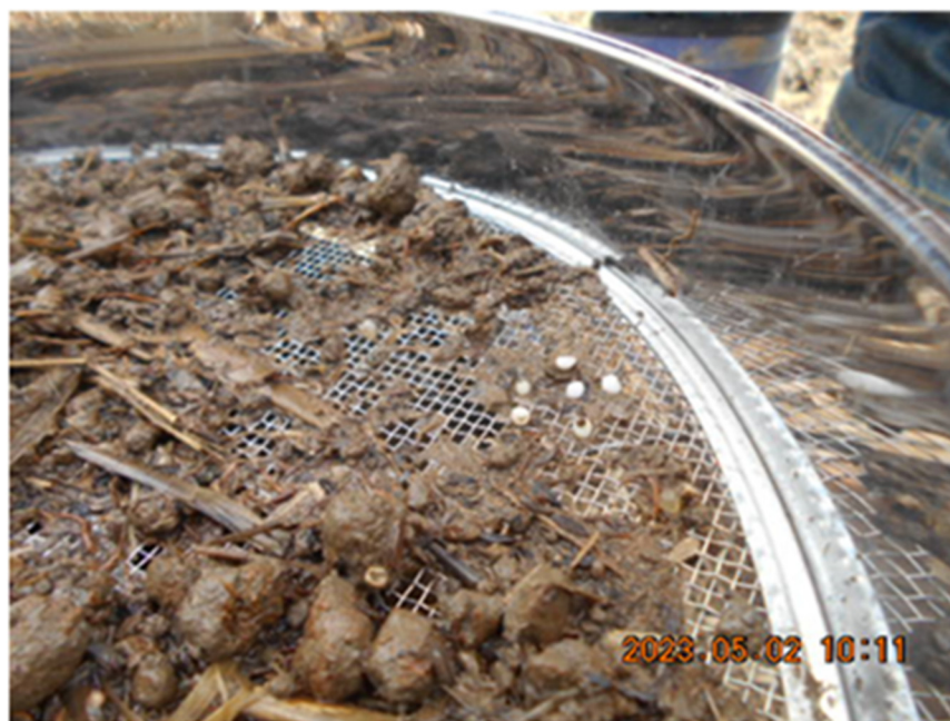
Figure 11. Washing a sample to remove soil and count the capsules in the sample.
