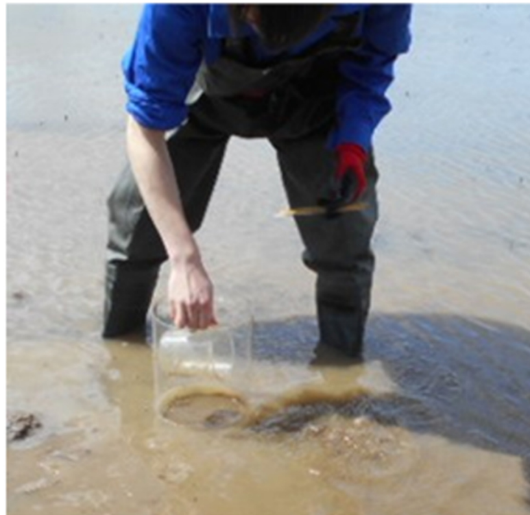
Figure 9. Insertion of an acrylic pipe into the paddy soil (to a depth of 15 cm) to collect fertilizer capsules.
