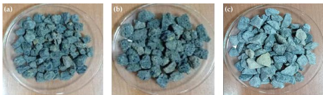
Figure 2. (a) Pozzolan with particle diameter of 3–6 mm; (b) Pozzolan with particle diameter of 7–9 mm; (c) Local gravel with particle diameter of 3–6 mm used as filter media.
