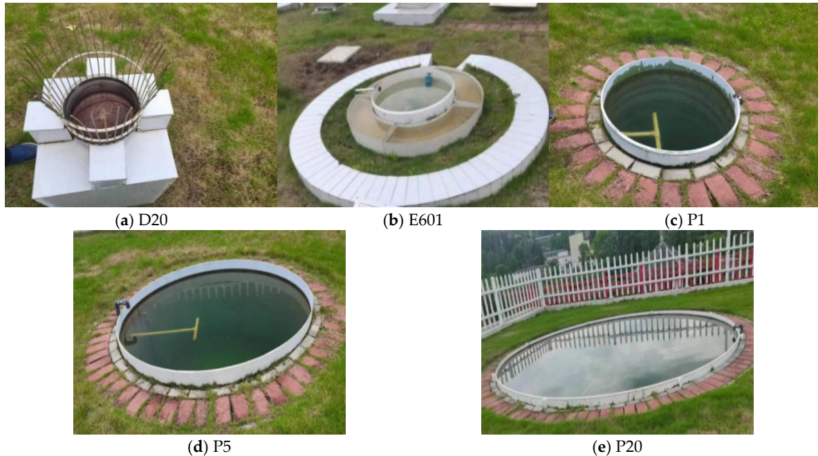
Figure 1. Illustration of five evaporation detection devices.
