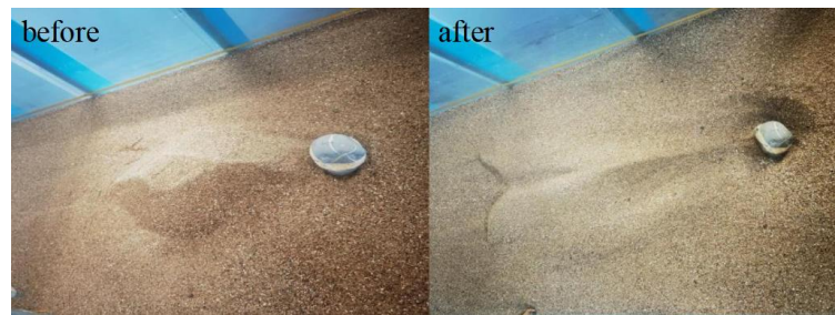
Figure 3. Bar scour processes with and without a boulder.
