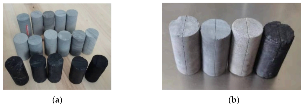
Figure 2. Representative photos of intact specimens and fractured specimens in permeability test. (a) Complete specimens. (b) Fractured specimens.
