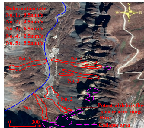
Figure 10. Early identification results of weak deformation in potential debris flow source areas.
