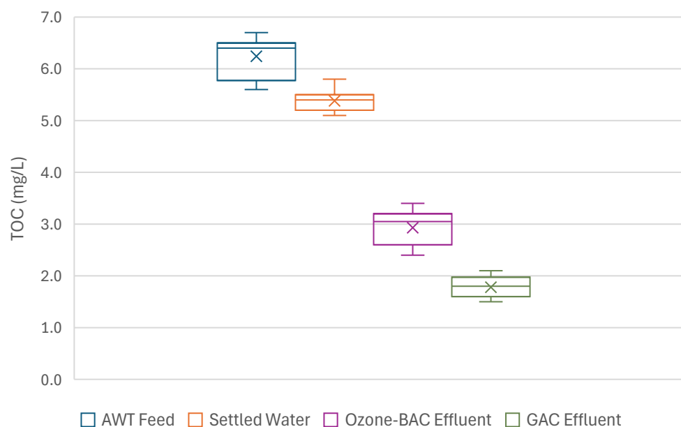
Figure 9. Substantial TOC removal occurred across the Pilot Study 2 treatment train. Data includes samples collected during challenge testing, following CFS and BAC optimization.
