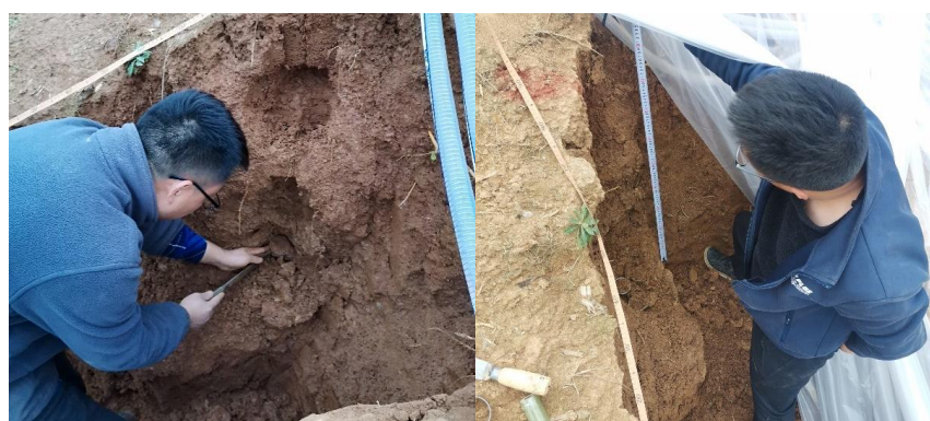
Figure 3. Undisturbed sample of ring cutter during test.
