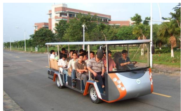
Figure 7: road test of solar and lithium-ion hybrid electric midibus
