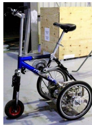
Figure 6: The prototype of the Man powered SEGWAY
