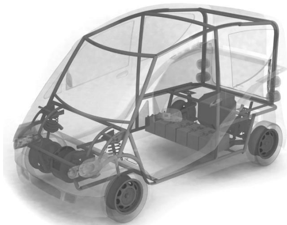
Figure 6: The ultra-light basket-tube frame vehicle designed and prototyped by Prof. Szumanowski's team
