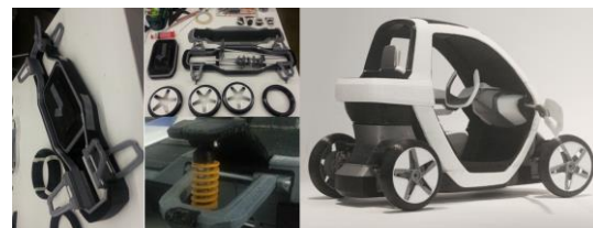
Figure 7: 3D-printed components and complete assembly
