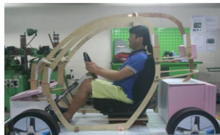
Figure 8: Ergonomics check using physical mock-up
