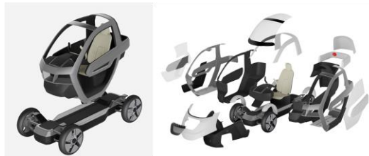
Figure 14: Modular design in vertical direction (left) and sub-modules of the body (right)
