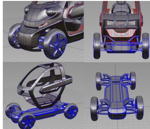
Figure 5: Block surfacing in the process of 3D digital modelling, showing complete assembly and components (Alias AutoStudio™)
