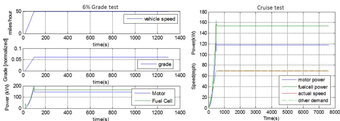
Figure 4. Power requirement for 6% grade at 50 mph and 70 mph cruise. 144 kW is required for the grade test and 118 kW for cruise test.
