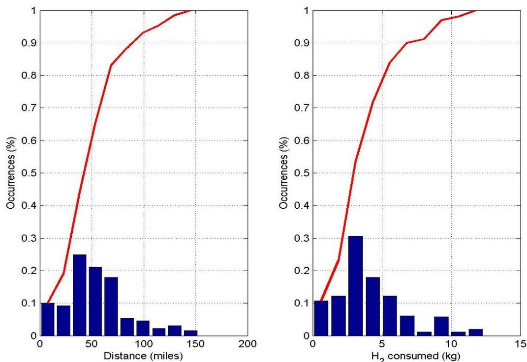
Figure 6. Performance of the Class 4 FCET on cycles from FleetDNA database. 150 mile range and 12 kg of Hydrogen is needed to satisfy all the driving conditions considered.
