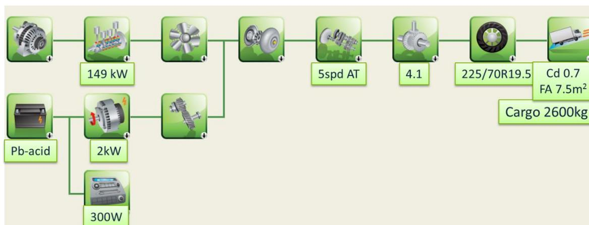
Figure 1. Schematic diagram for a conventional medium duty vehicle. Component specifications are also shown.
