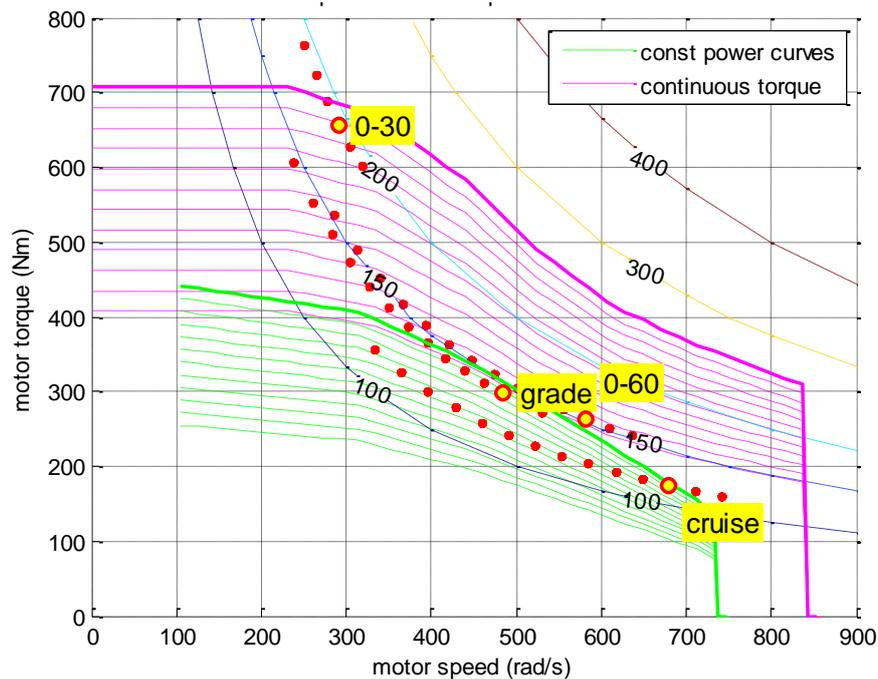
Figure 5. Finding an appropriate motor power and the overall speed reduction ratio.
