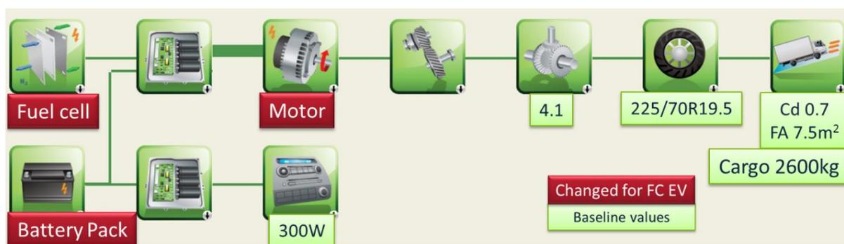
Figure 2. Schematic diagram for a medium duty fuel cell electric truck.
