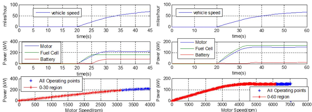
Figure 3. Acceleration power requirement of motor is estimated at 224 kW for the FCET to achieve 0-30 mph in 7.2 s (left) and 154 kW motor output power is sufficient for accelerating from 0-60 mph in 29.8 s (right).
