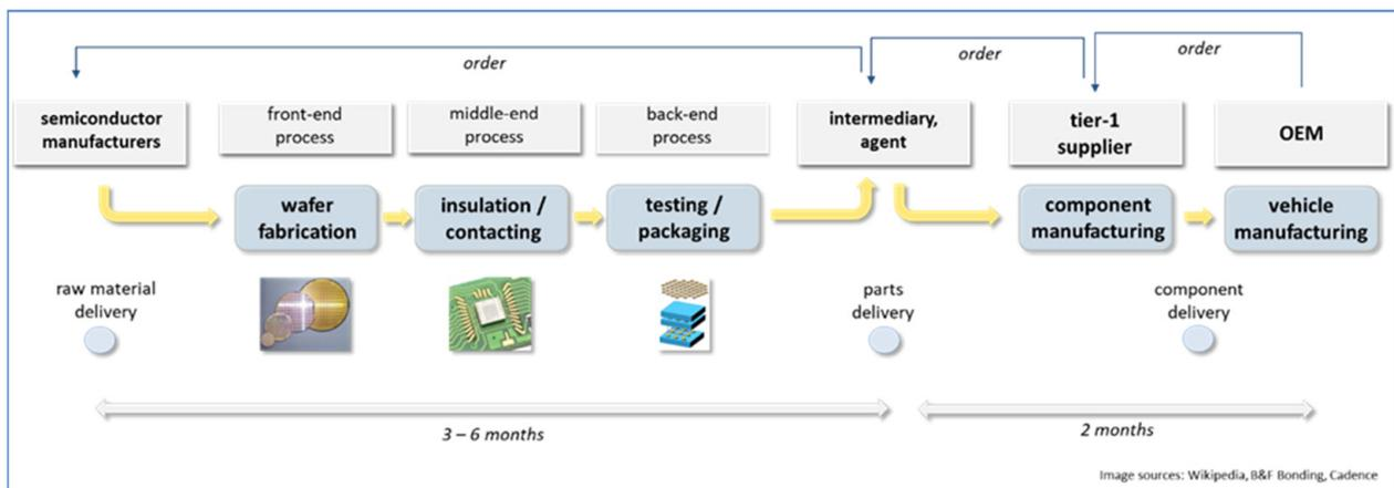
**Figure 4.** Production and supply chain for semiconductor components [18].
