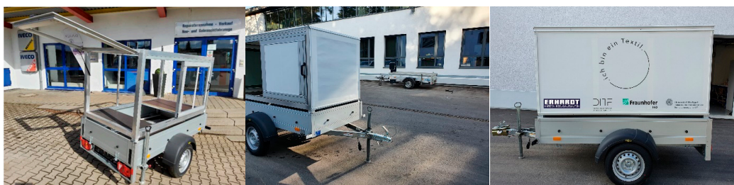
Figure 12. Final prototype of the textile vehicle body at a trailer.
