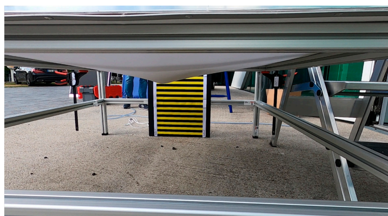
Figure 11. Example of recording the drift punch of a package in front of the reference scale.
