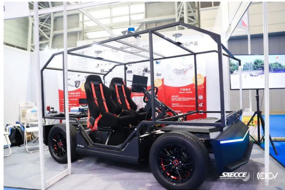
**Figure 1.** Teemo four-wheel steering intelligent chassis.
