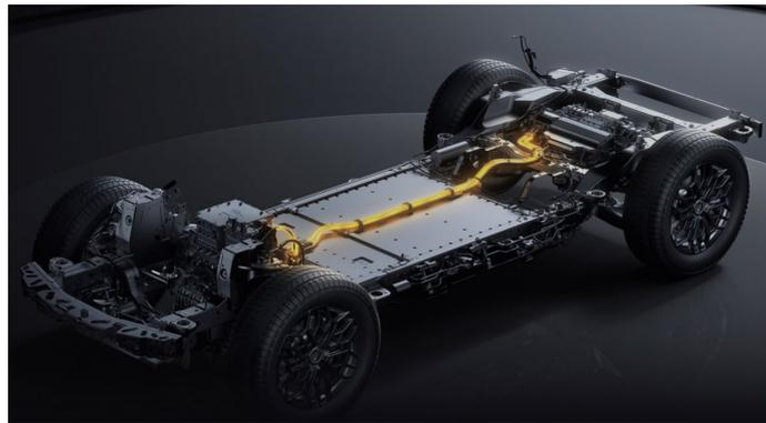
**Figure 2.** Yang Wang U8 distributed drive chassis.
