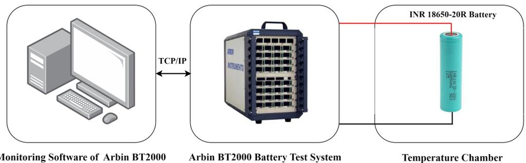
Figure 5. Experimental setup for battery tests [69].
