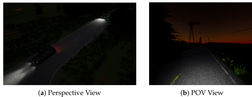
Figure 3. Low-Illumination Scenario where vehicle in front is not visible in RGB camera.
