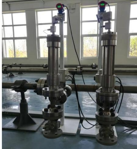
Figure 11. Real-time phase content monitoring sampler
