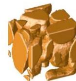
Optimized pore structure based on CT scan and; below: estimated velocity profiles from lattice Boltzmann flow
