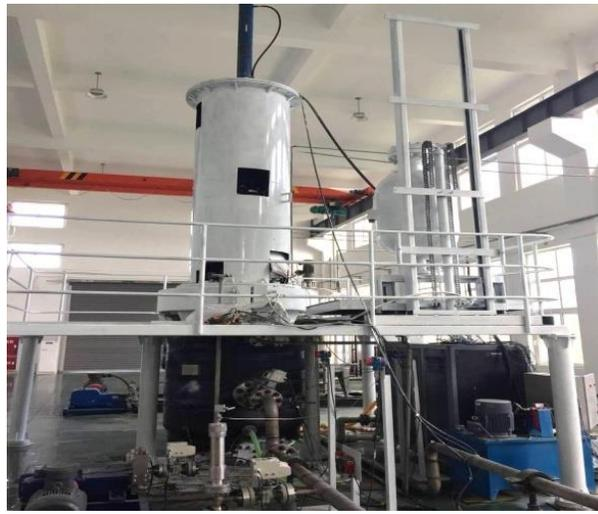
Figure 7. Preparing and breaking system of the hydrate
